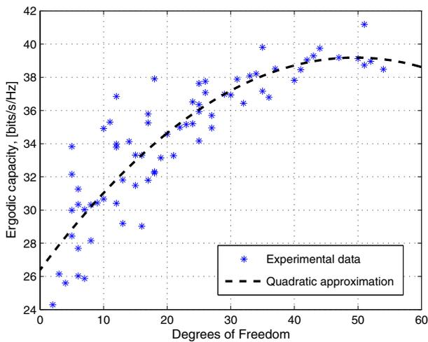
**Fig. 3.** Ergodic capacity,  $\bar{C}$ , against the spatial DoF,  $D$  ( $\rho = 20$  dB).
