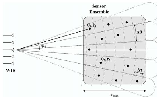
Figure 1: Active Wireless Sensing: basic communication architecture.
