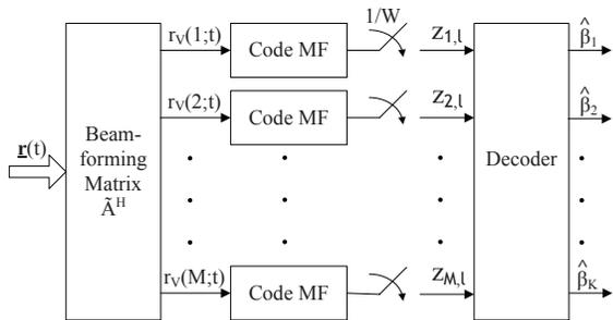
**Figure 2: Computation of sufficient statistics at the WIR: angle-delay matched filtering.**
