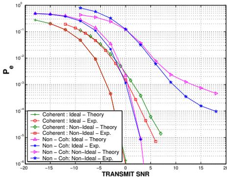
**Figure 5: Comparison of analytical  $P_e$  calculations with numerical results.**
