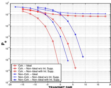
**Figure 6:  $P_e$  versus SNR plot for high-rate information retrieval with interference suppression. 121 bits per transmission.**
