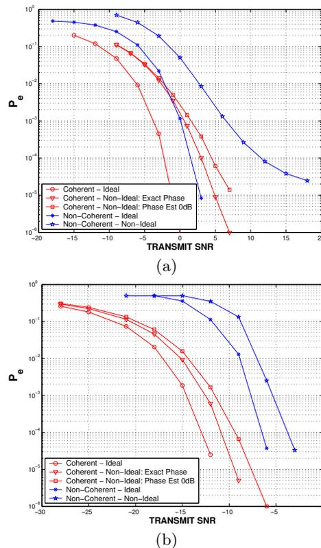
**Figure 4:  $P_e$  vs. SNR plots. (a) Independent sensor transmissions. 11 bits per transmission. (b) Identical sensor transmissions. 1 bit per transmission.**
